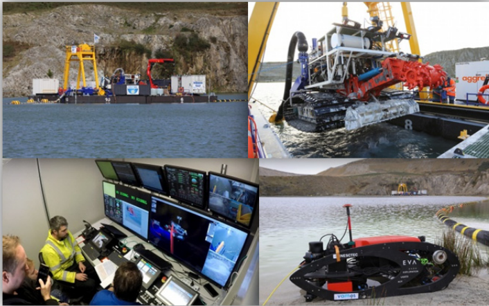
iVAMOS! Underwater mining machine, exploration iVAMOS! AUV [EVA] and real time monitoring interface in the control station.
