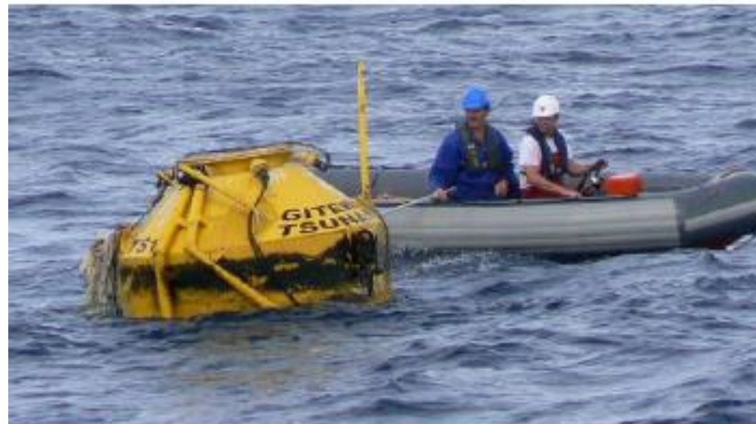
Figure 16. Australian Tsunameter - Stolen Superstructure and Electronics Payload
