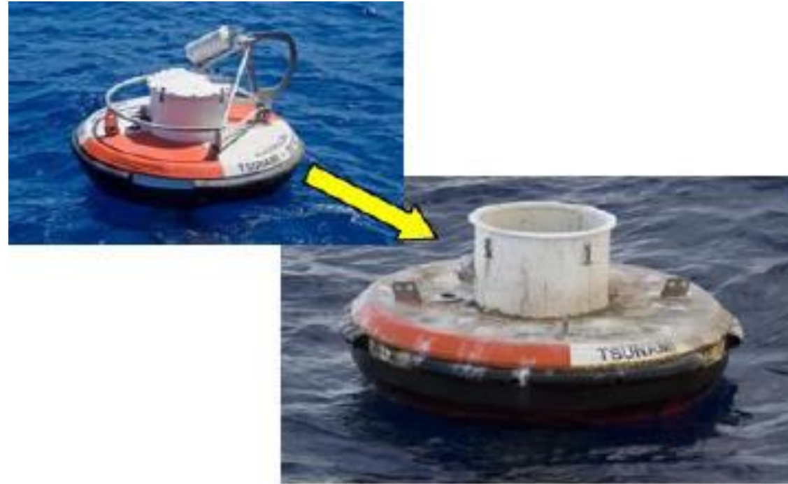
Figure 16. Australian Tsunameter - Stolen Superstructure and Electronics Payload
