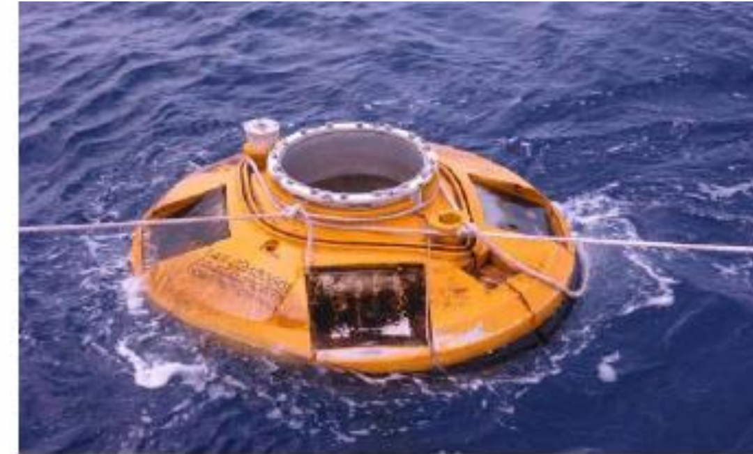
Figure 17. Indian Tsunami Buoy – Stolen Superstructure and Electronics Payload
