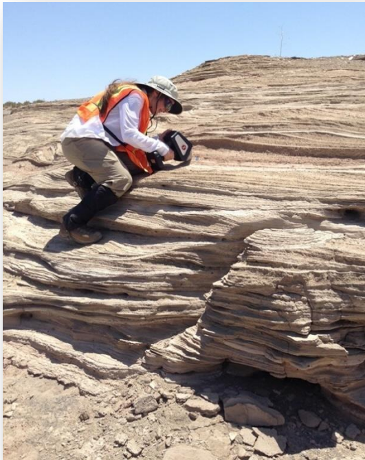
Amy using the handheld LIBS at a field site in the Portillo Volcanic Field, New Mexico, USA.
