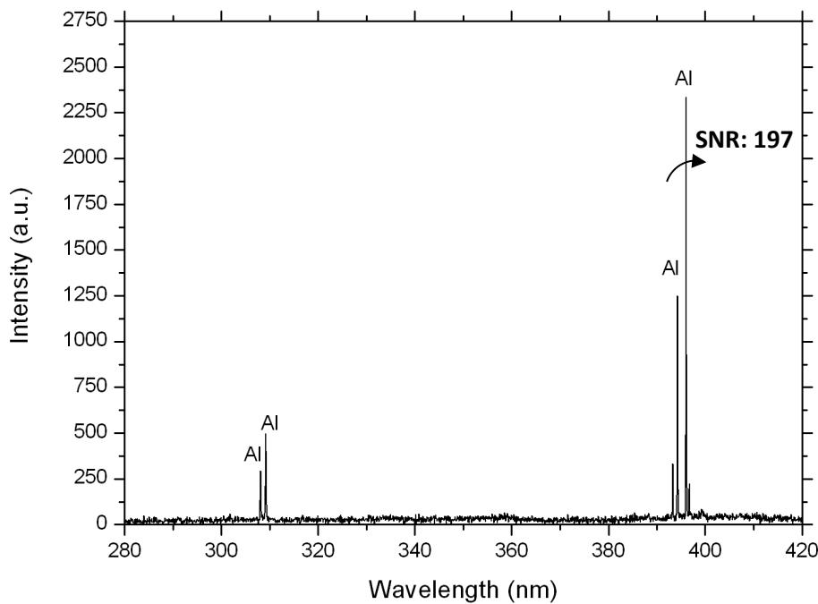
**Al<sub>2</sub>O<sub>3</sub> particle – 100 nm
