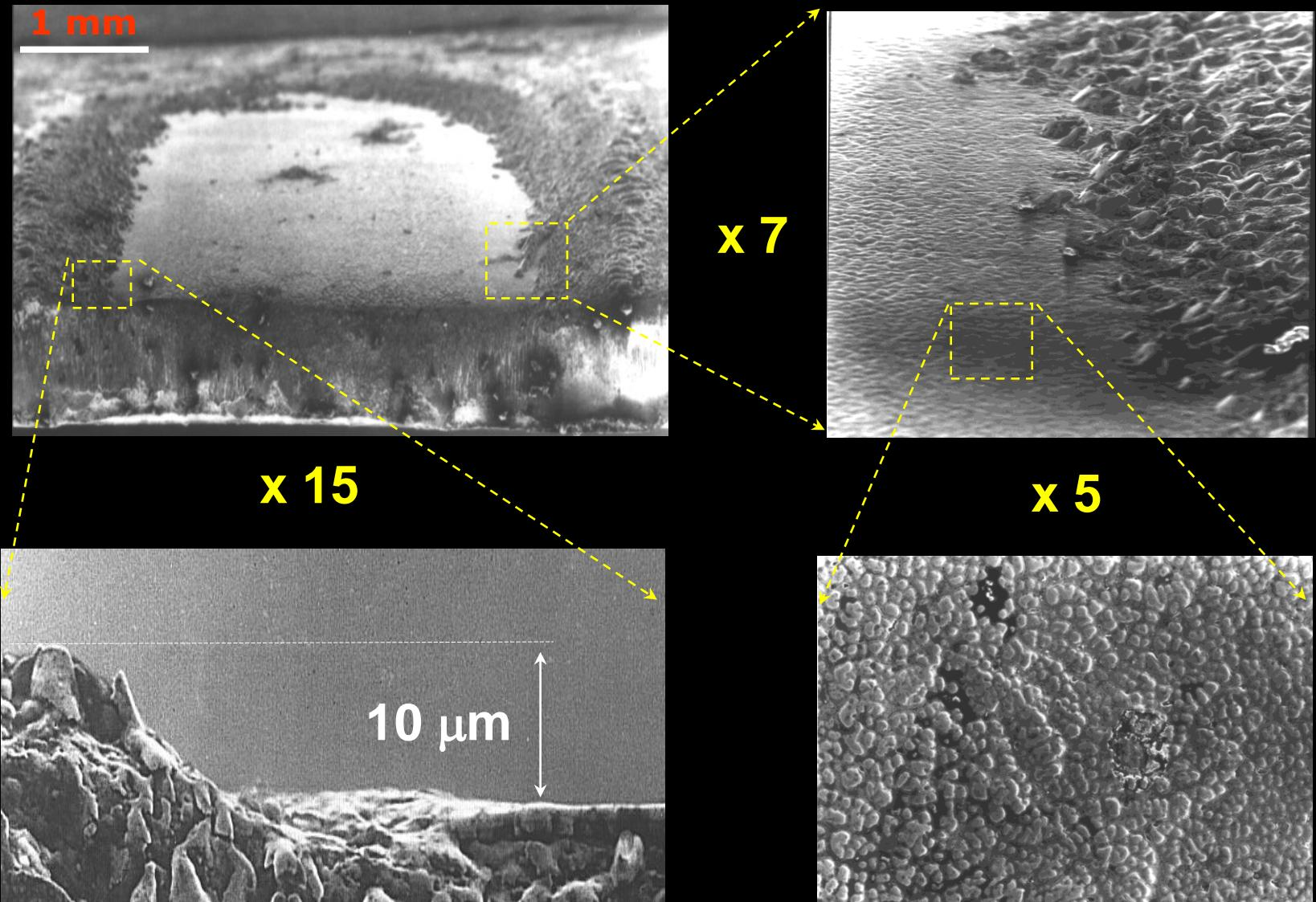
Zn-coated steel; 4000 pulses XeCl (308 nm);
